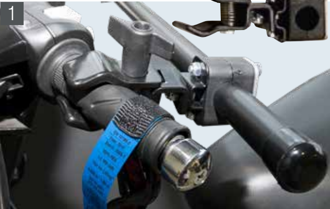
Fastening the holding arm to the handlebars with a cross clamp
