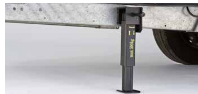
Support automatically extends telescopically
