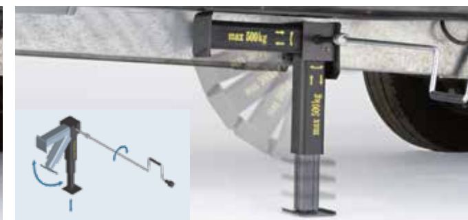
Crank until the stand is on the floor
