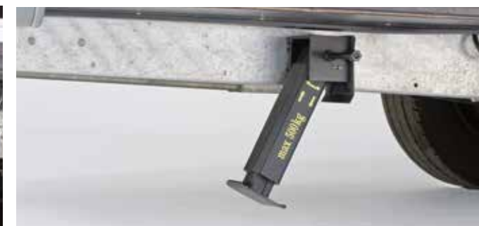
Crank until support is in vertical position
