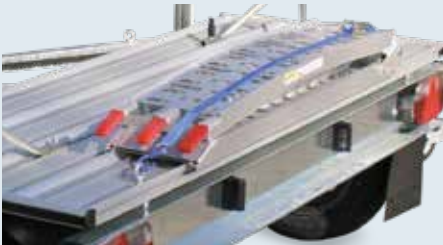
Folding access ramp. Loadable up to 340 kg.
