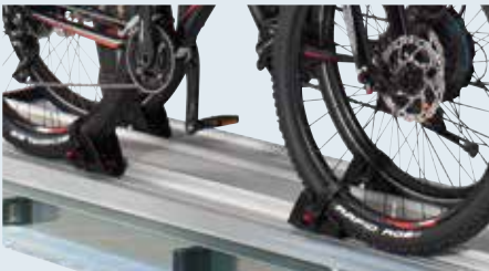
Wheel shells with ratchet quick-release fastener for bicycles.
